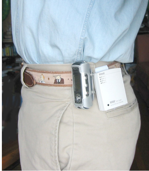
Figure 1: Data capture equipment. In the middle of the picture is the iRiver flash memory recorder. The larger unit to the right is a data logger recording ambient temperature, which we have considered as a proxy for more specific ground truth on location changes.
