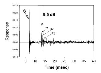
FIG. 1. The recording of the response to a  $10-\mu s$  electrical pulse in a college classroom that was approximately  $6 \times 11$  m in size. The source of the transient was placed 1.3 m in front of a blackboard attached to the front of the classroom and the recording was made 4 ft in front of the source. The first 40 ms of the recording shows the direct click (*S*) and several early reflections labeled as *R*1, *R*2, and *R*3. These reflections stand out from the overall reverberation.
