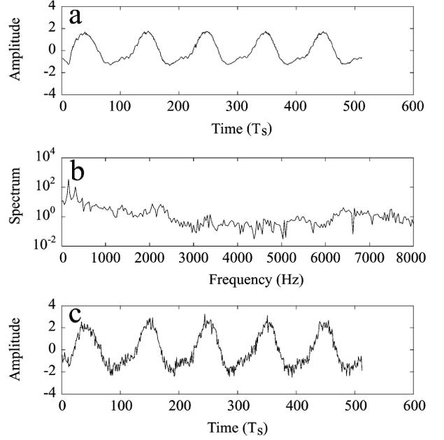
Fig. 1. Signals used for the simulation: (a) source signal  $s(t)$ , (b) source spectrum,  $|S(f)|$ , (c) the simulated measurement  $x(t) = s(t - T_s) + 0.5s(t - 8.75T_s) + n(t)$ , where  $T_s = 62.5 \mu\text{s}$  is the sample interval and  $n(t)$  is varying levels of ambient noise.
