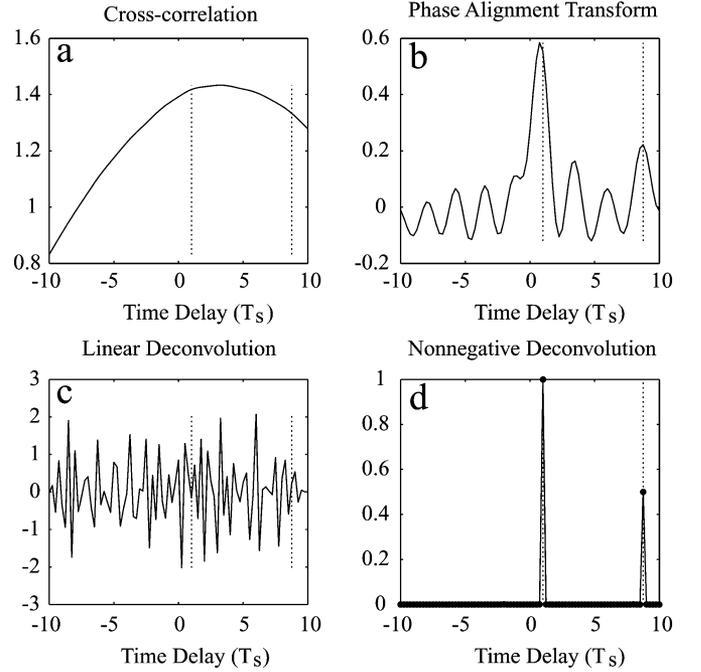
Fig. 2. Time-delay estimation of the room impulse response  $h(t) = \delta(t - T_s) + 0.5\delta(t - 8.75T_s)$  by (a) cross correlation, (b) phase alignment transform, (c) linear deconvolution, and (d) nonnegative deconvolution. The vertical dotted lines in each plot indicate the true positions of the time delays  $\Delta t = T_s$  and  $\Delta t = 8.75T_s$ , respectively.
