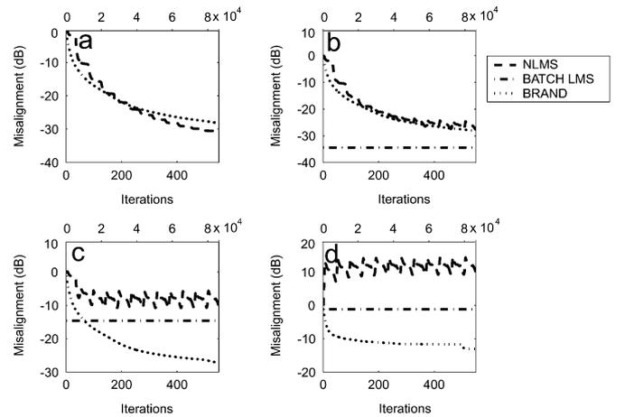
Fig. 7. Normalized misalignment of NLMS (dashed line), batch LMS (dashed-dotted line), and BRAND (dotted line) with varying levels of added noise: (a) no noise; (b)  $-40$  dB; (c)  $-20$  dB; and (d)  $0$  dB. The horizontal axes indicate the number of iterations for BRAND (lower axis) and NLMS (upper axis). Batch LMS led to zero misalignment when the signal had no noise.
