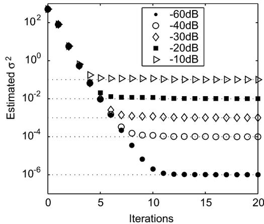
Fig. 3. Estimate of  $\sigma^2$  at each iteration of the BRAND algorithm for signals with varying levels of noise. Uniform regularization was employed for the first ten iterations, followed by another ten iterations of independent regularization.
