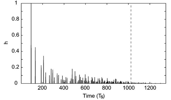
Fig. 6. Room impulse response derived from image model with parameters shown in Table I. The first 1024 samples were used in the simulation.
