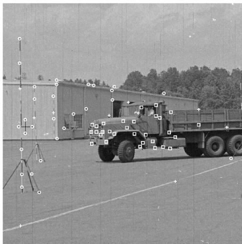
Fig. 14. Results of MMGLR. The motion group corresponding to the truck is denoted by squares, and the motion group corresponding to the background is denoted by circles. The detected outliers are shown as "+" signs.
