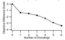
Figure 1. Effect of multiple encodings on audio quality. The Objective Difference Grade measures perceived difference in quality between a reference and test signal.
