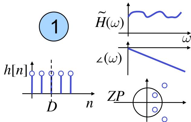
$$\begin{aligned} H(e^{j\omega}) &= \sum_{n=0}^N h[n]e^{-j\omega n} \\ &= e^{-j\omega\frac{N}{2}} \left( h\left[\frac{N}{2}\right] + 2 \sum_{n=1}^{N/2} h\left[\frac{N}{2}-n\right] \cos \omega n \right) \end{aligned}$$
