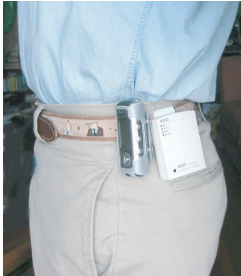
Figure 1.1: Data capture equipment. In the middle of the picture the iRiver flash memory recorder. The larger unit to the right is a data logger recording ambient temperature, which we have considered as a proxy for more specific ground truth on location changes.
