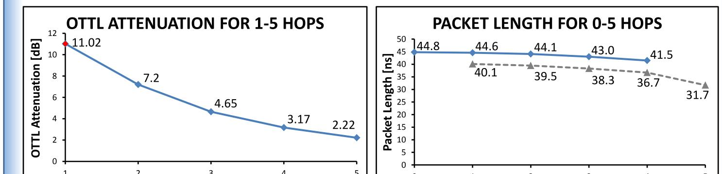
As Attenuation Is Reduced From  $\lambda_{OTTI}$ , The Optical Packet Travels More Hops Through The Buffer
