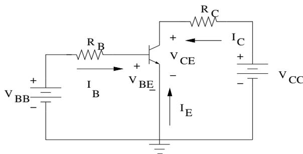
Figure 1: A Common Emitter circuit employing an *npn* transistor
