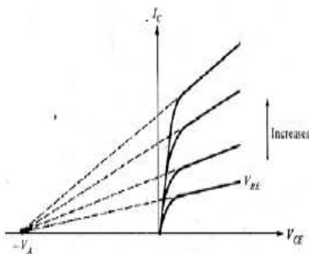
Figure 3: Common-emitter output characteristics for an npn transistor with  $V_{BE}$  as a parameter. The curves are extended back (dashed lines) to the negative  $V_{CE}$  axis and intersect as the Early voltage
