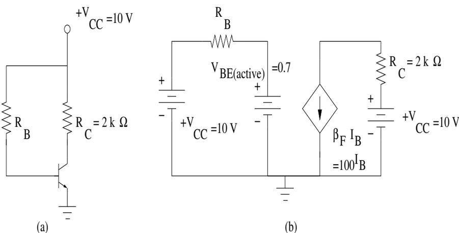
Figure 6: (a) Schematic diagram of the CE configuration; (b) equivalent circuit of the part (a)
