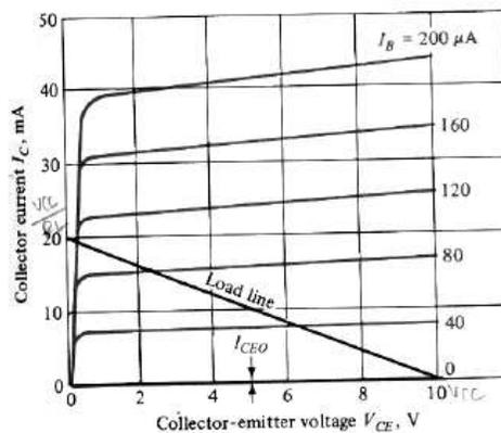
Figure 2: A Common Emitter output characteristics of *npn* transistor. A load line is superimposed
