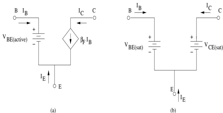
Figure 5: Large-signal (dc) equivalent circuits for an *npn* transistor for (a) forward-active and (b) saturation-region operation
