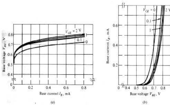
Figure 4: (a) Common-emitter input characteristics ( $V_{BE}$  versus  $I_B$ ) for the 2N2222A transistor; (b) the curves in part a plotted as  $I_B$  versus  $V_{BE}$ . Note the similarity with the diode characteristic.
