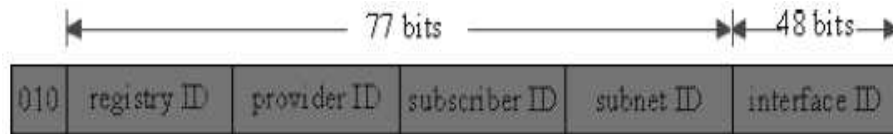
Figure 3.10: IPv6 address format
