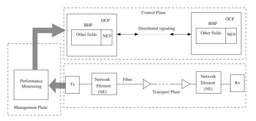
Fig. 1. Structure of the control plane for the distributed signaling.
