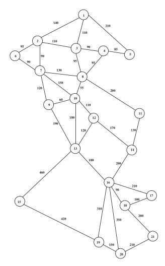
Fig. 6. Topology for Italian high-capacity network, consisting of 21 nodes and 36 bidirectional links.
