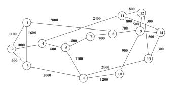
Fig. 5. Network topology of NSF network, consisting of 14 nodes and 21 bidirectional fiber links.
