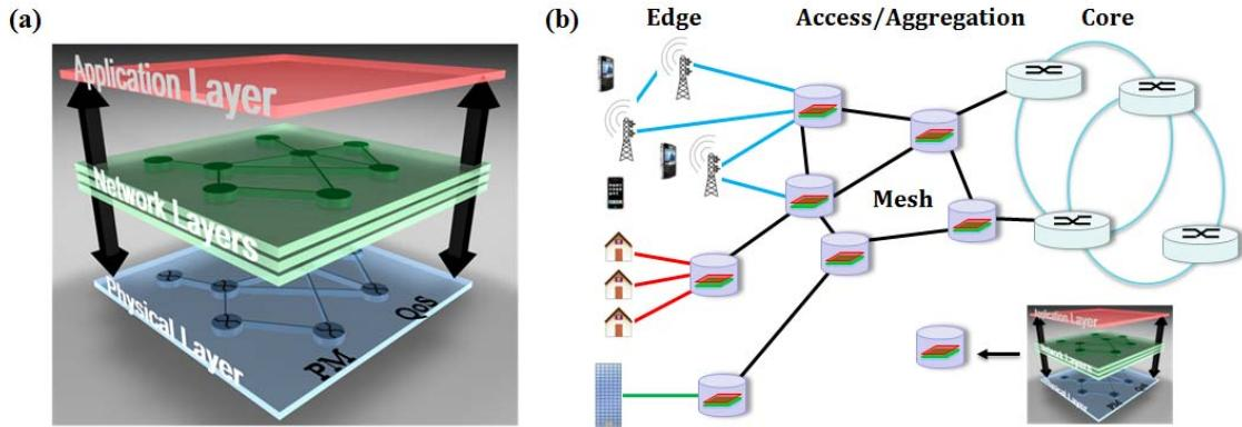
Figure 1: (a) Cross-layer optimized network protocol stack, with physical-layer awareness of the higher network layers; (b) Block diagram of the mesh-centred design to interconnect the cross-layer nodes.
