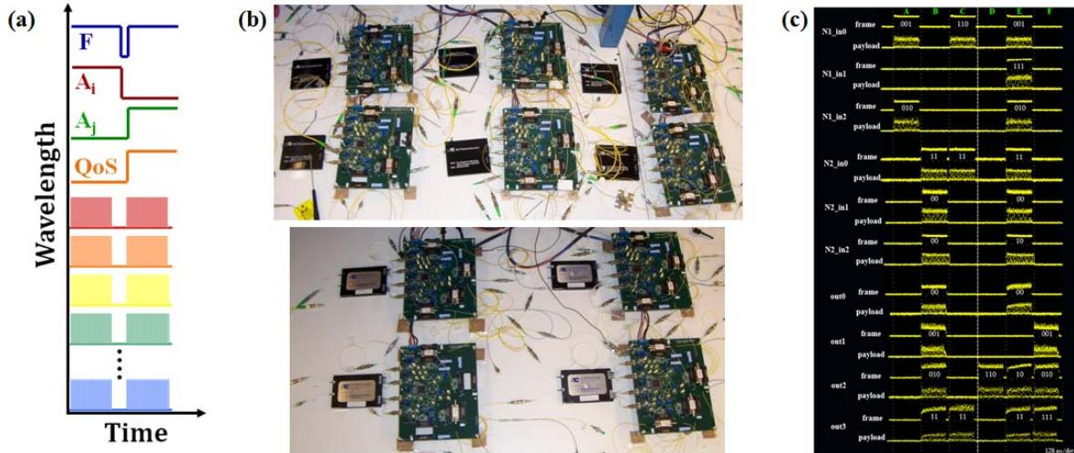
Figure 3: (a) Wavelength-striped packet format; (b) Photograph of multicast-capable switching fabric test-bed; (c) Experimental waveform traces of the input and output optical traffic, with labels referring to the address information encoded in the optical packets.
