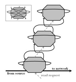
**Fig. 1.** The buffer's cascade structure (large image). A  $3 \times 3$  non-blocking switch, of which a reduced version is used to implement the modules (inset) [9]
