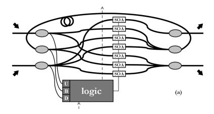
Fig. 2. Schematic diagram of the building-block module with ovals for couplers; U, B, and D for their respective low-speed receivers; dashed lines for read request signals [9]
