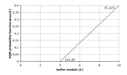
**Fig. 3.** The AQM dropping-probability function, defined by  $x_1$  and  $y_2$ . In this case  $x_1 = 4, y_2 = 0.4$  and the buffer capacity is C = 10.
