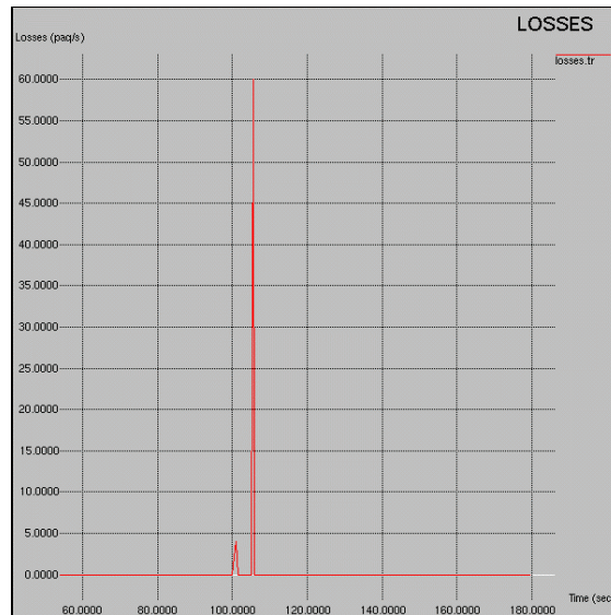
Figure 3: Packets of VoIP Traffic Lost per Second when De-coupled.
