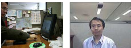
Figure 1. Basic system setup. The camera is placed on top of the computer screen or on another location facing the user. A microphone is also placed near the screen to capture voice activity.
