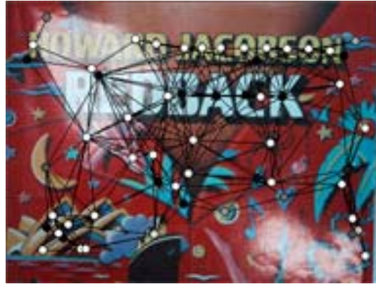
Figure 4.10. Output from the pairwise MRF model (brightness of nodes represents the probability as “text”)
