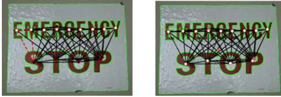
Figure 4.6. (Left) The miss in detecting multiple text lines due to cross-text-line (CTL) cliques. (Right) the results after potential function modification.
