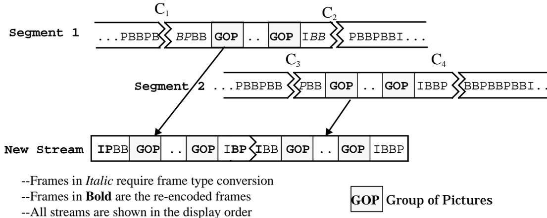
FIGURE 1. Cut and Paste MPEG bitstreams in the compressed domain.
