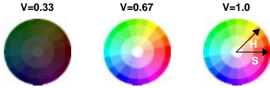
FIGURE 3. Quantized HSV color space, 18 hues, 3 saturations and 3 values + 4 grays = 166 colors.
