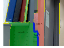
Fig. 2. Sample segmentation results by NCuts. A thickened boundary segment is shown to indicate the potential splicing boundary.
