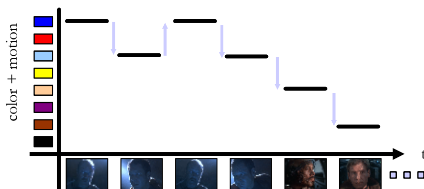
Figure 2.1: A shot detector based on color and motion, segments the video into piece-wise constant approximations with respect to the two features.
