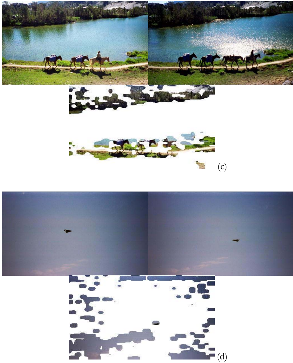
Figure 67. Example of change areas obtained by the block-based correlation algorithm.
