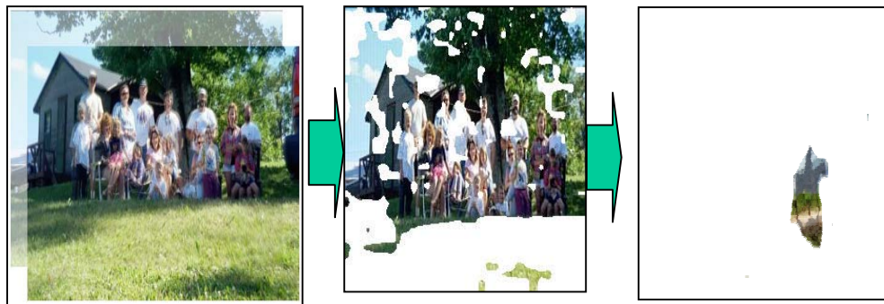
Figure 63. Three basic steps in our framework: (1) alignment, (2) detection of change areas, (3) local analysis of change areas.
