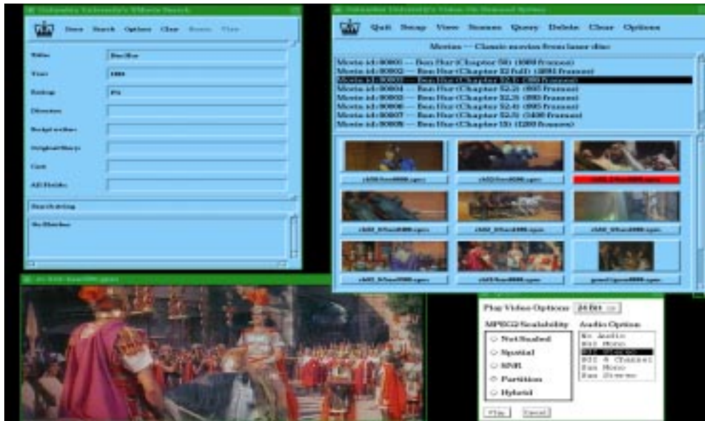
FIGURE 3. Current user interface of Columbia University's VOD tested. This snapshot shows the video scene browser, the MPEG-2 playback interface, the QoS setup panel, and the bibliographic search database.
