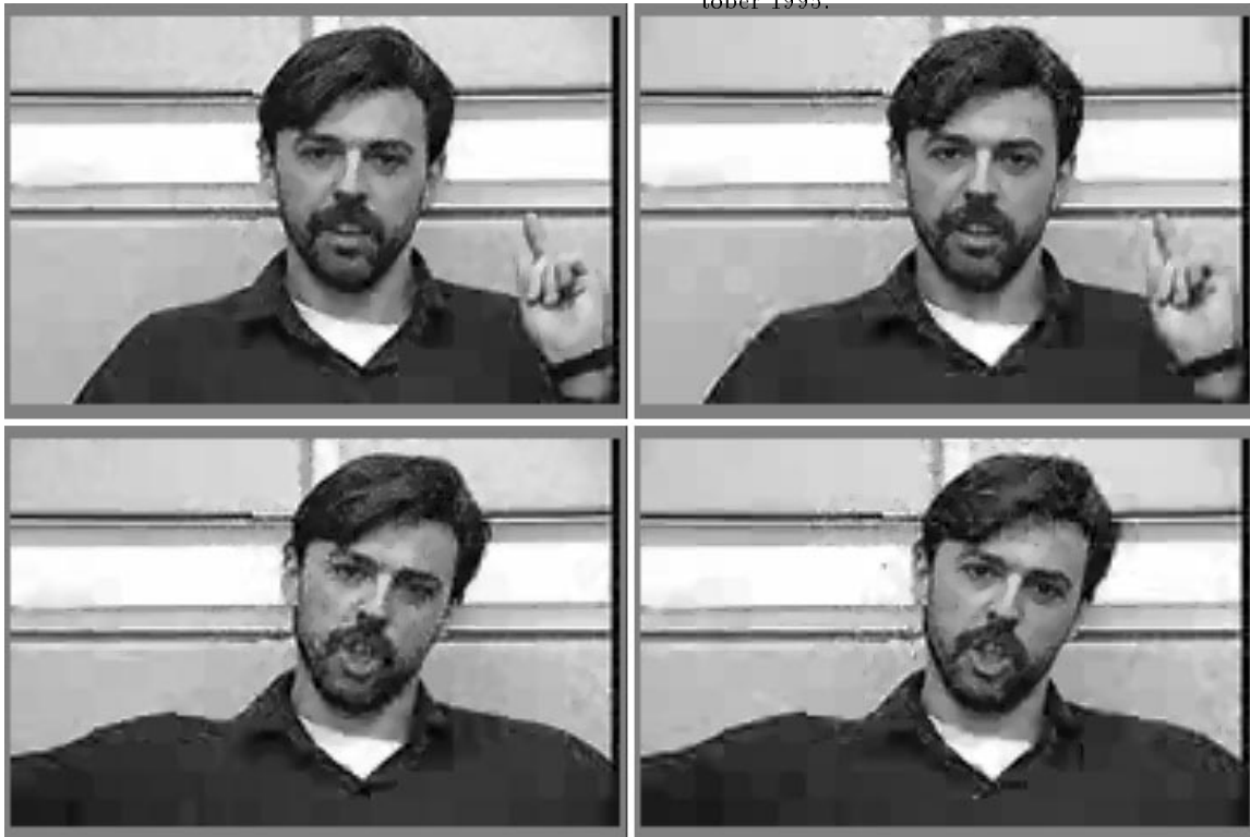
Figure 4: Stills from sequence “roberto” coded at 48 kbps, 5 fps, with RM8 (left), and Model-Assisted RM8 (right).
