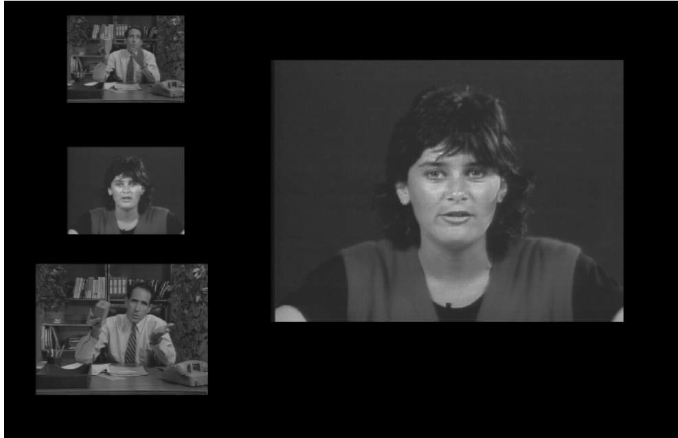
Fig. 6. A typical compositing scenario in video conferencing. The input images are scaled down with different ratios and translated to different positions. The image shown is reconstructed from the compressed output which is composited in the DCT domain. The input images are compressed with MC+DCT.
