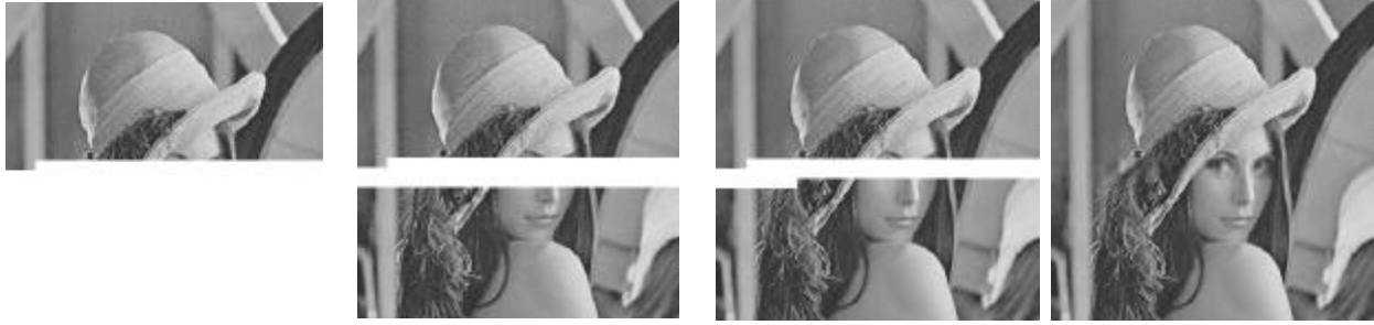
Figure 6: Effects of packet loss in a JPEG bitstream: (a) without reset (RST) marks, (b) with RST marks, after resynchronization.
