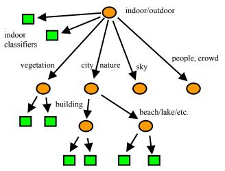
**Figure 4:** A Bayesian network for consumer photographs. It integrates multiple classes (circles) and classifiers (squares) using different media. Note the number of classifiers for each class can be arbitrary. Each link is associated with conditional probabilities modeling the dependence between the parent and the child class.
