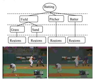
**Figure 5**. A multi-level scene model for the pitching scene in baseball. The bottom part shows a test baseball image and its segmented image map as the input to the multi-level classifier.
